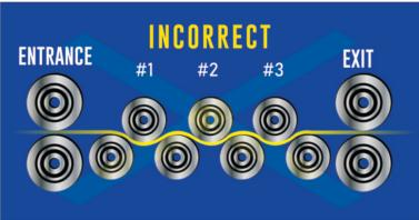
The Straghtener is designed to remove coil set. The general rule for steel strips is that the exit setting should be set to strip thickness, and the entry setting should be somewhat deeper. "Approximately 30%–50% of material thickness". Starting with these initial adjustments, make finer adjustments until the product is flat as it emerges from the machine. If the strip has an upward curvature, then the exit setting must be decreased, or vice versa.
