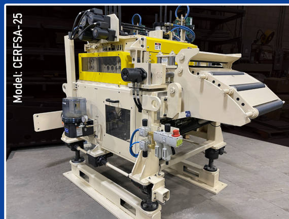
Alligator Head Servo Feeder-Straightener Combo
